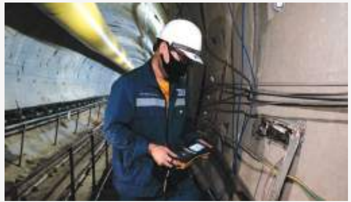
Total Pressure Cell Monitoring in Tunnel
